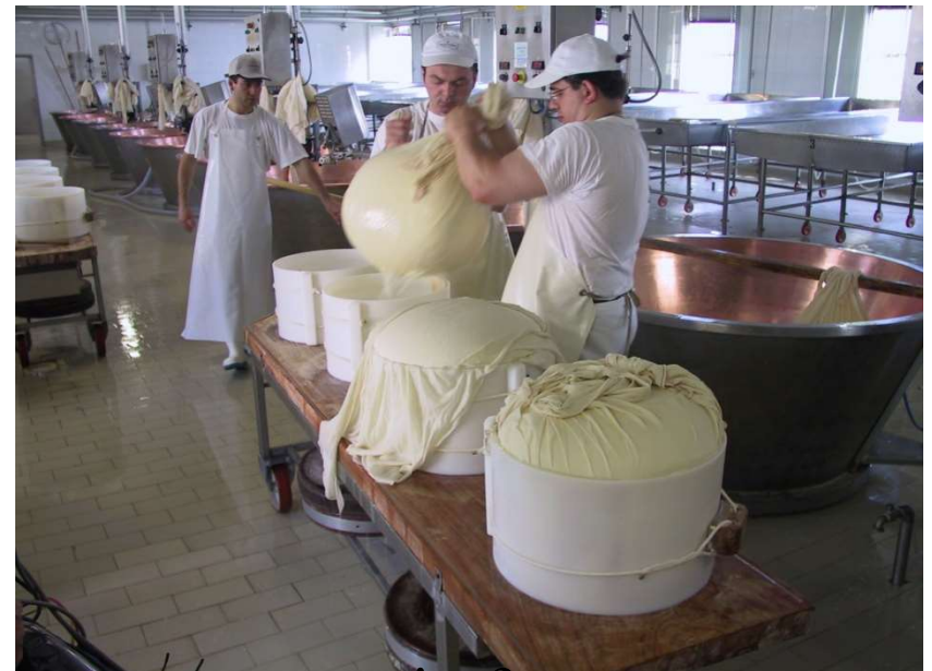
messa in fascera
